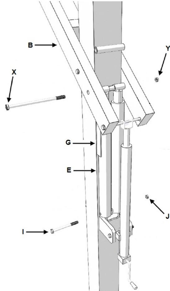
Lower the system to relieve the pressure on your blue spring assist spacer and then remove it.
