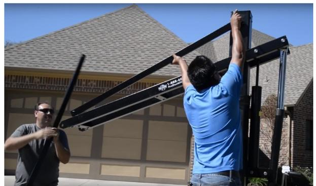
**NOTE:** It does not matter which end of the parallel link you attach to the vertical post.
