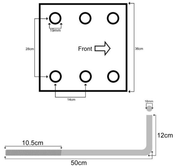
Use the level to ensure that the pier anchor template (G) it is level in all directions. Additionally, the center line of the 18mm Anchor J-Bolts (H) must be parallel with the edge of the playing surface.
